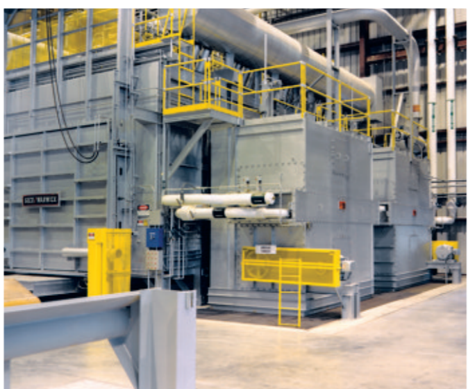
Bypass cooler reduces fin maintenance and keeps performance at peak levels
